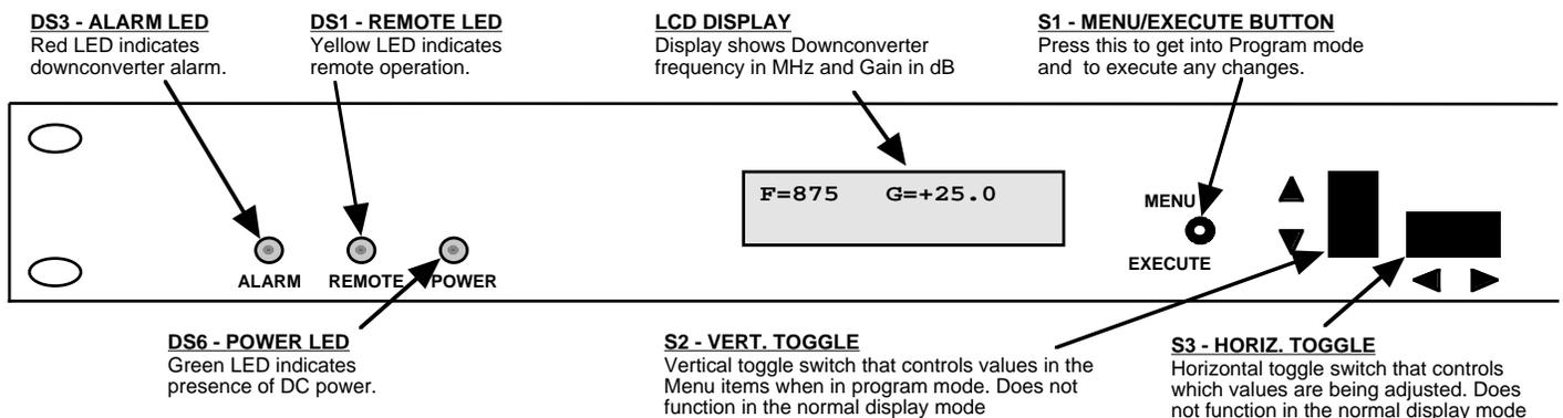
**FIGURE 2.3 2016-10 Front Panel Controls and Indicators**
