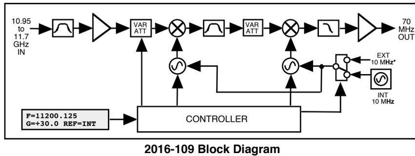
**FIGURE 1.2 Model 2016-109 Downconverter Block Diagram**
