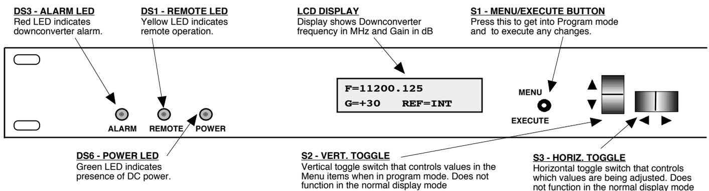
**FIGURE 2.3 2016-109 Front Panel Controls and Indicators**
