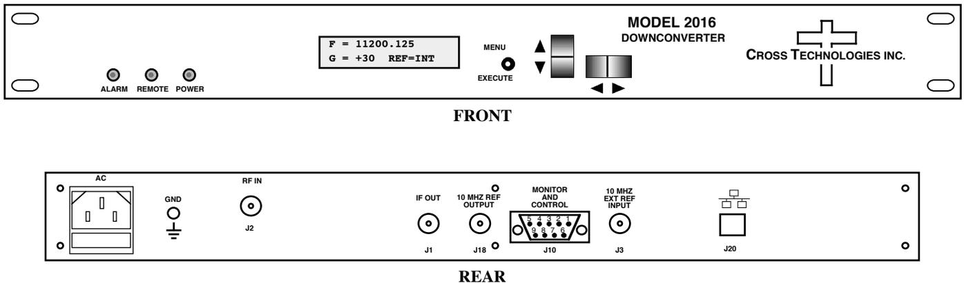
**FIGURE 1.1 Model 2016-109 Front and Rear Panels**
