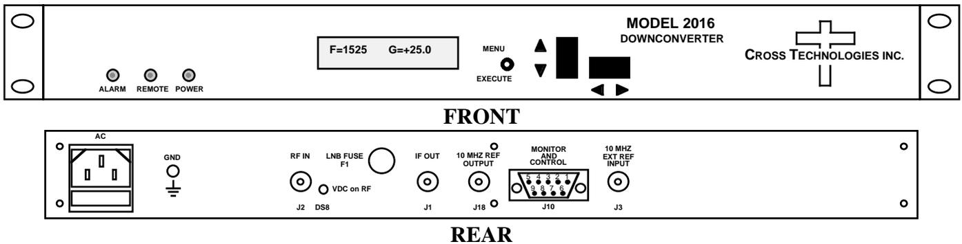
**FIGURE 1.1 Model 2016-05 Front and Rear Panels**
