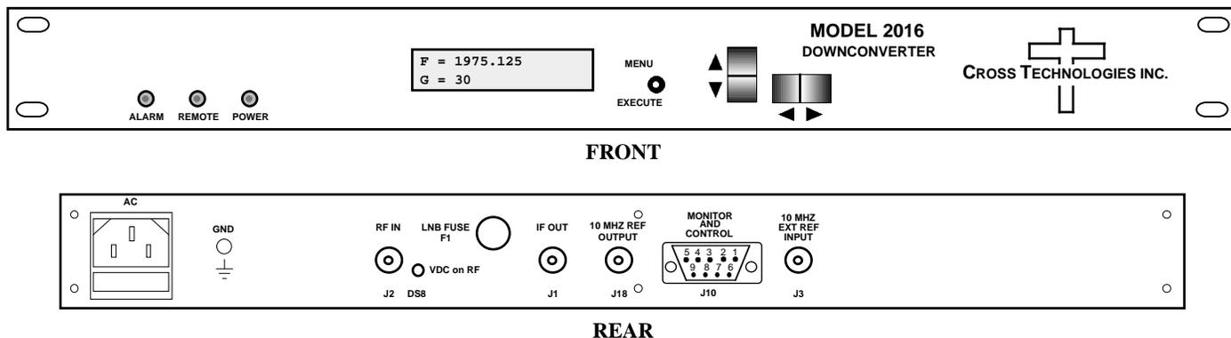
**FIGURE 1.1 Model 2016-02-370 Front and Rear Panels**
