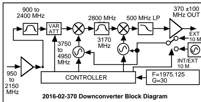
**FIGURE 1.2 Model 2016-02-370 Downconverter Block Diagram**
