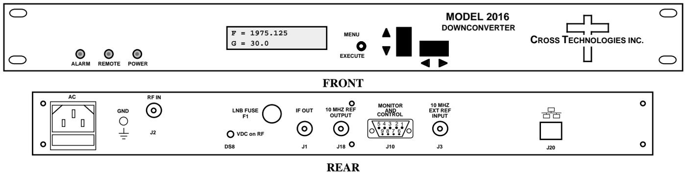
**FIGURE 1.1 Model 2016-02-720-400 Front and Rear Panels**
