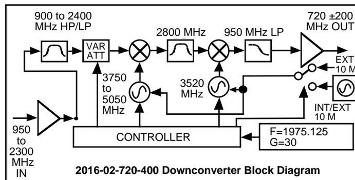
**FIGURE 1.2 Model 2016-02-720-400 Downconverter Block Diagram**
