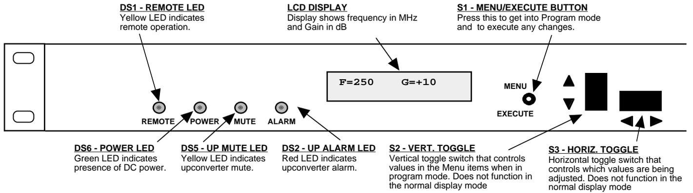
**FIGURE 2.2 2015-75 Front Panel Controls and Indicators**
