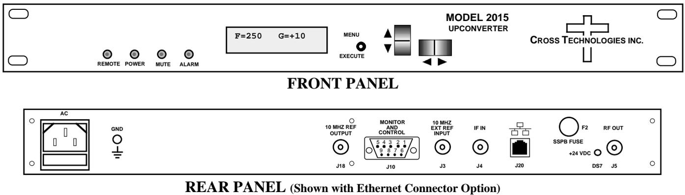
**FIGURE 1.1 Model 2015-75 Front and Rear Panels**
