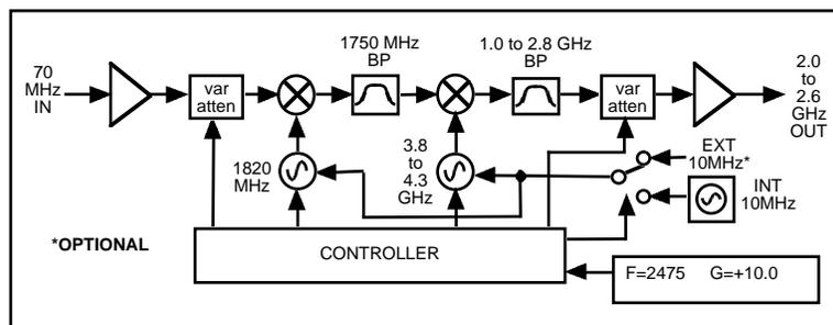
**FIGURE 1.2 Model 2015-2026 Upconverter Block Diagram**
