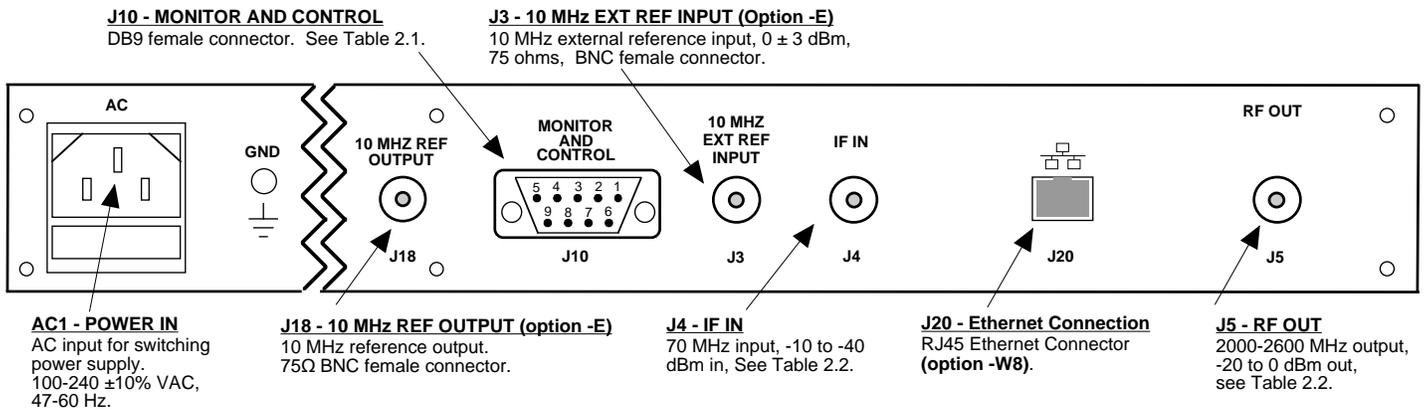
**FIGURE 2.2-A 2015-2026 Rear Panel I/Os - AC Input**
