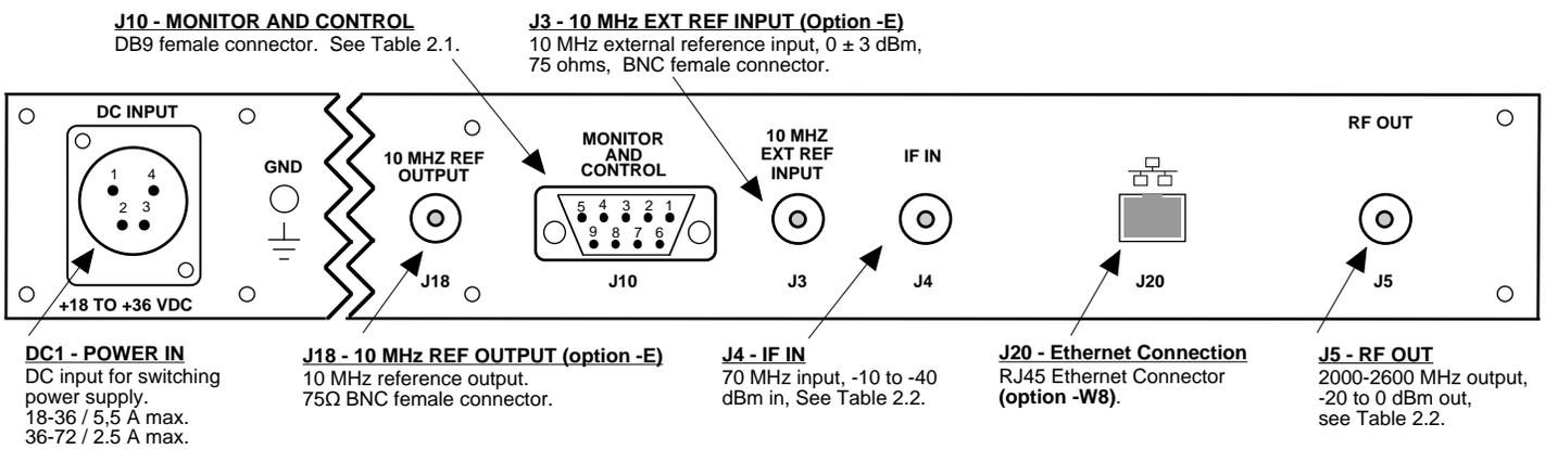
**FIGURE 2.2-B 2015-2026 Rear Panel I/Os - DC Input**
