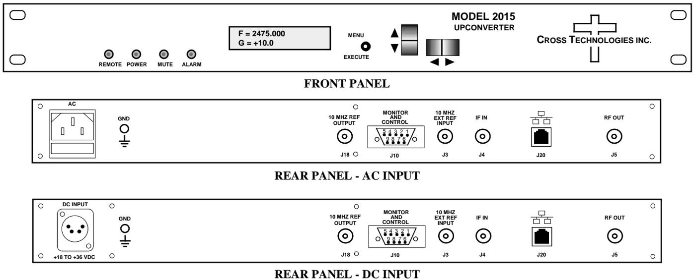
**FIGURE 1.1 Model 2015-2026 Front and Rear Panels**
