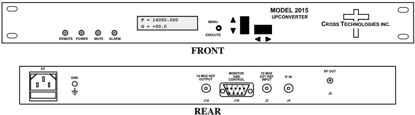
**FIGURE 1.1 Model 2015-145 Front and Rear Panels**
