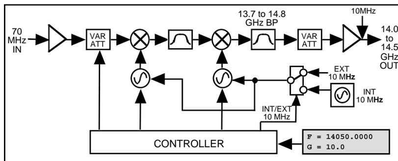
**FIGURE 1.2 Model 2015-145 Upconverter Block Diagram**
