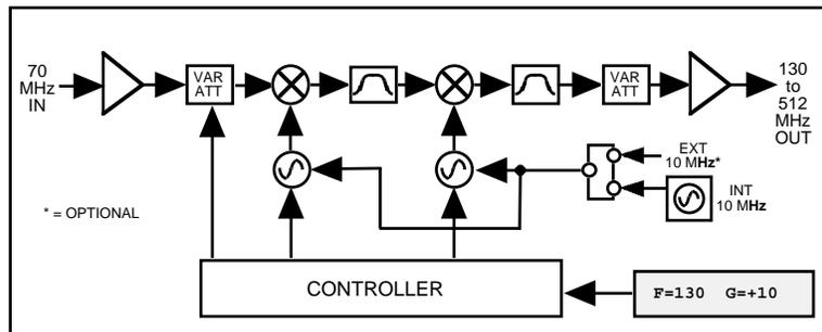
**FIGURE 1.2 Model 2015-1351 Upconverter Block Diagram**
