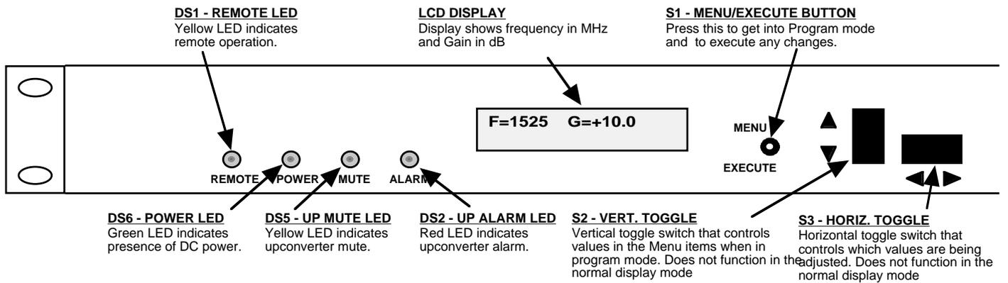
**FIGURE 2.2 2015-05 Front Panel Controls and Indicators**
