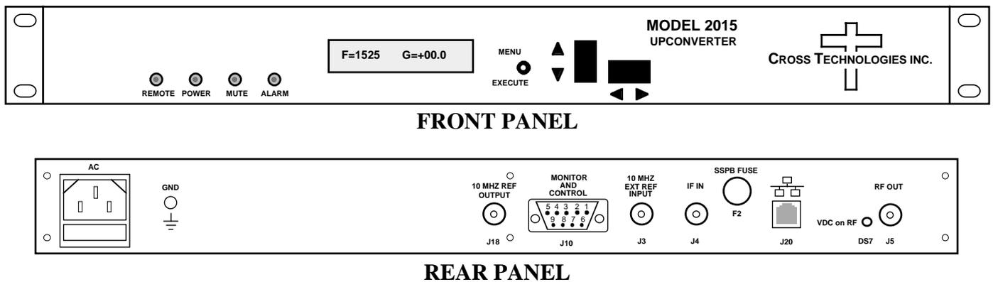
FIGURE 1.1 Model 2015-02 Front and Rear Panels
