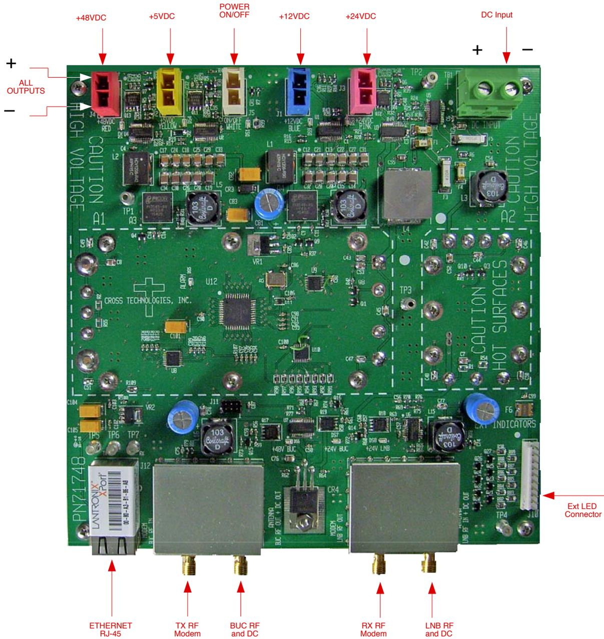
**FIGURE 2.2 Top View Connections**
