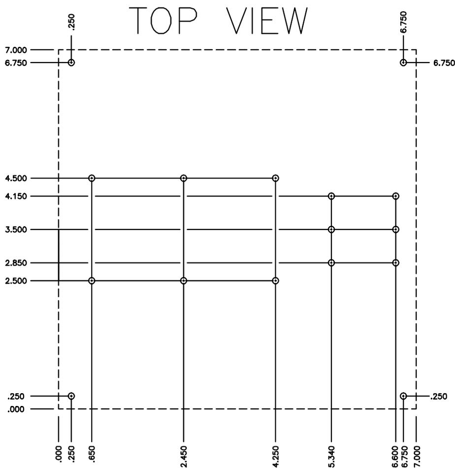
**FIGURE 2.1 Power Supply Mounting Pattern**
