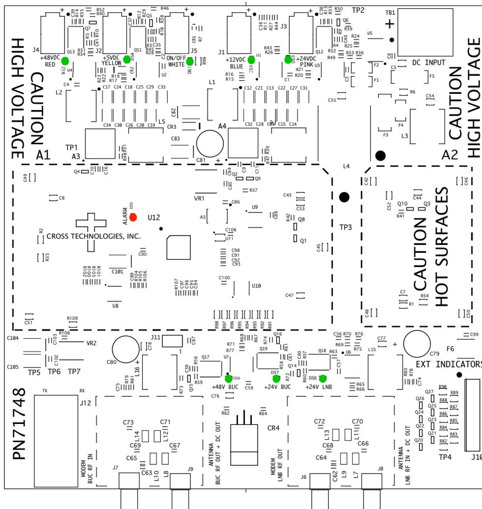
FIGURE 1.1 TOP VIEW - Showing Onboard Indicators (Shown with W90 and W92 Options)
