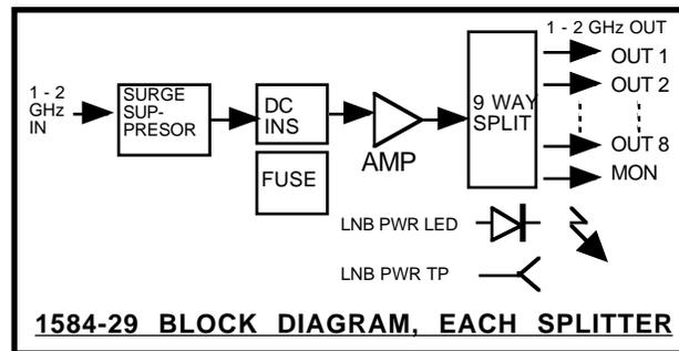
**FIGURE 1.2 MODEL 1584-29 RF SPLITTER BLOCK DIAGRAM**
