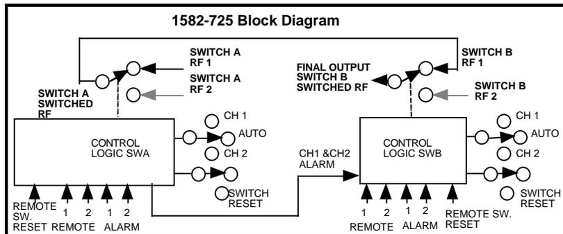
**FIGURE 1.2 Model 1582-725 RF Switch Block Diagram (Each Switch)**
