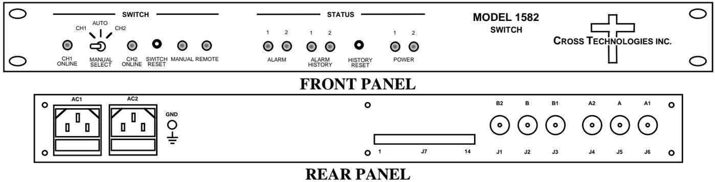
**FIGURE 1.1 Model 1582-22L Front and Rear Panels**
