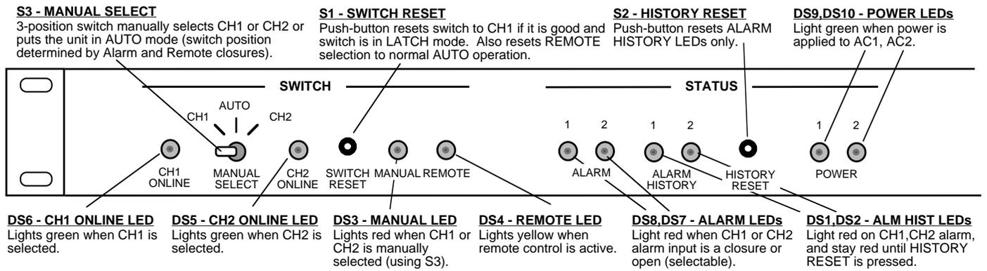
**FIGURE 2.3 1582-22L Front Panel Controls and Indicators**
