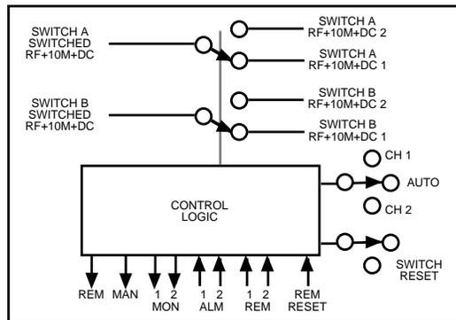
**FIGURE 1.2 Model 1582-22L RF Switch Block Diagrams**
