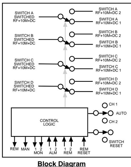
FIGURE 1.2 Model 1582-22L2 RF Switch Block Diagrams
