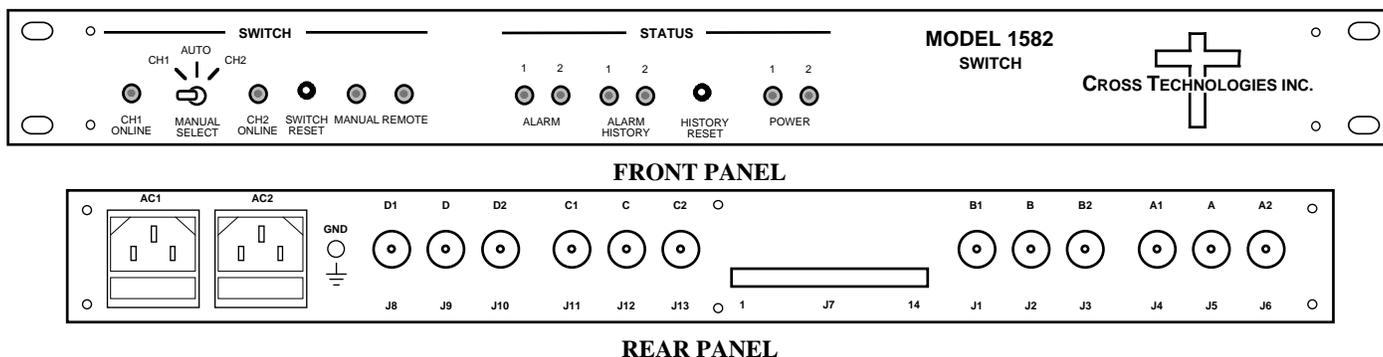
FIGURE 1.1 Model 1582-22L2 Front and Rear Panels
