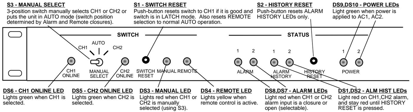
**FIGURE 2.3 1582-22L2 Front Panel Controls and Indicators**
