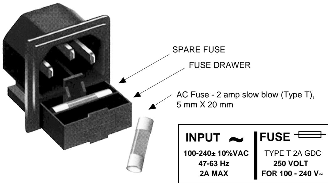
**FIGURE 2.4** Fuse and Spare Fuse Locations
