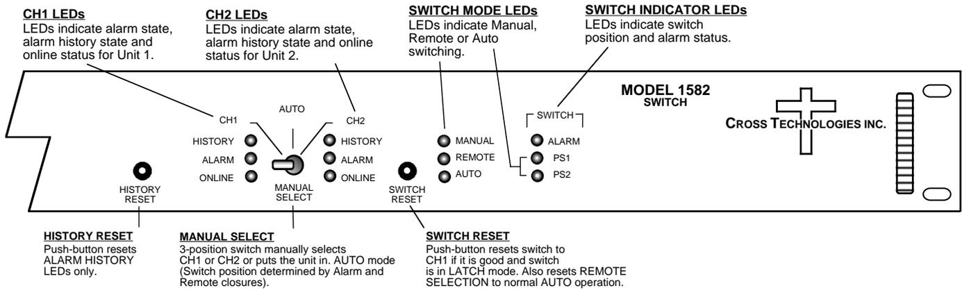
**FIGURE 2.3** 1582-122L Switch, Front Panel Controls and Indicators
