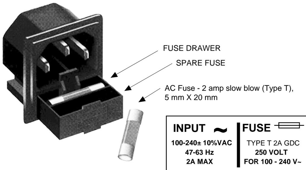
**FIGURE 2.4 Fuse and Spare Fuse Locations**
