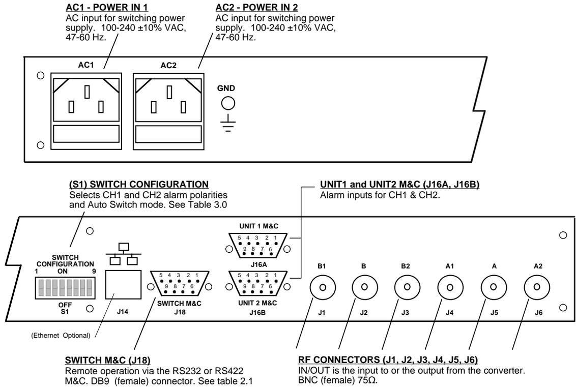
**FIGURE 2.2 1582-122L Switch Rear Panel Inputs/Outputs**
