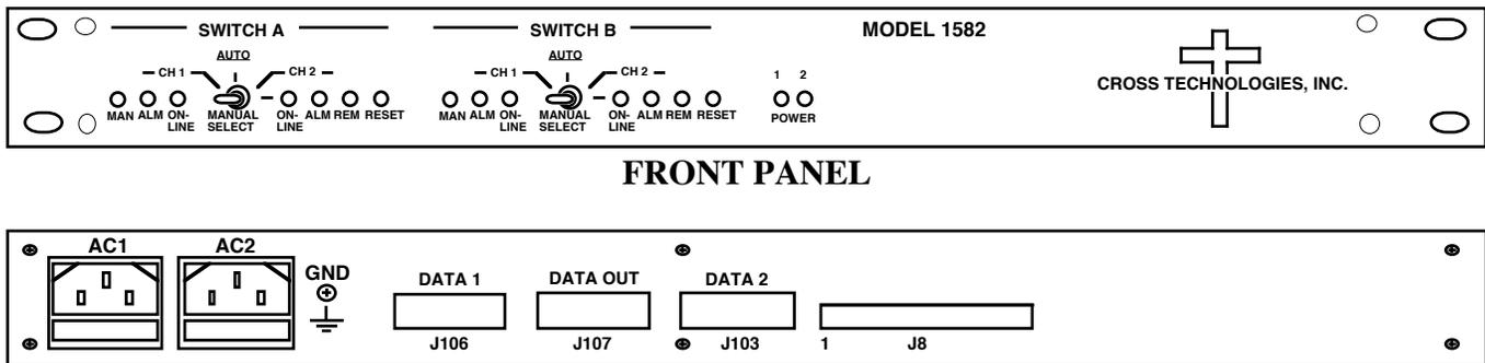
**FIGURE 1.1 Model 1582-03 Front and Rear Panels**
