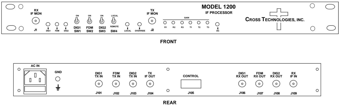
**FIGURE 1.1 Model 1200-04 Front and Rear Panels**
