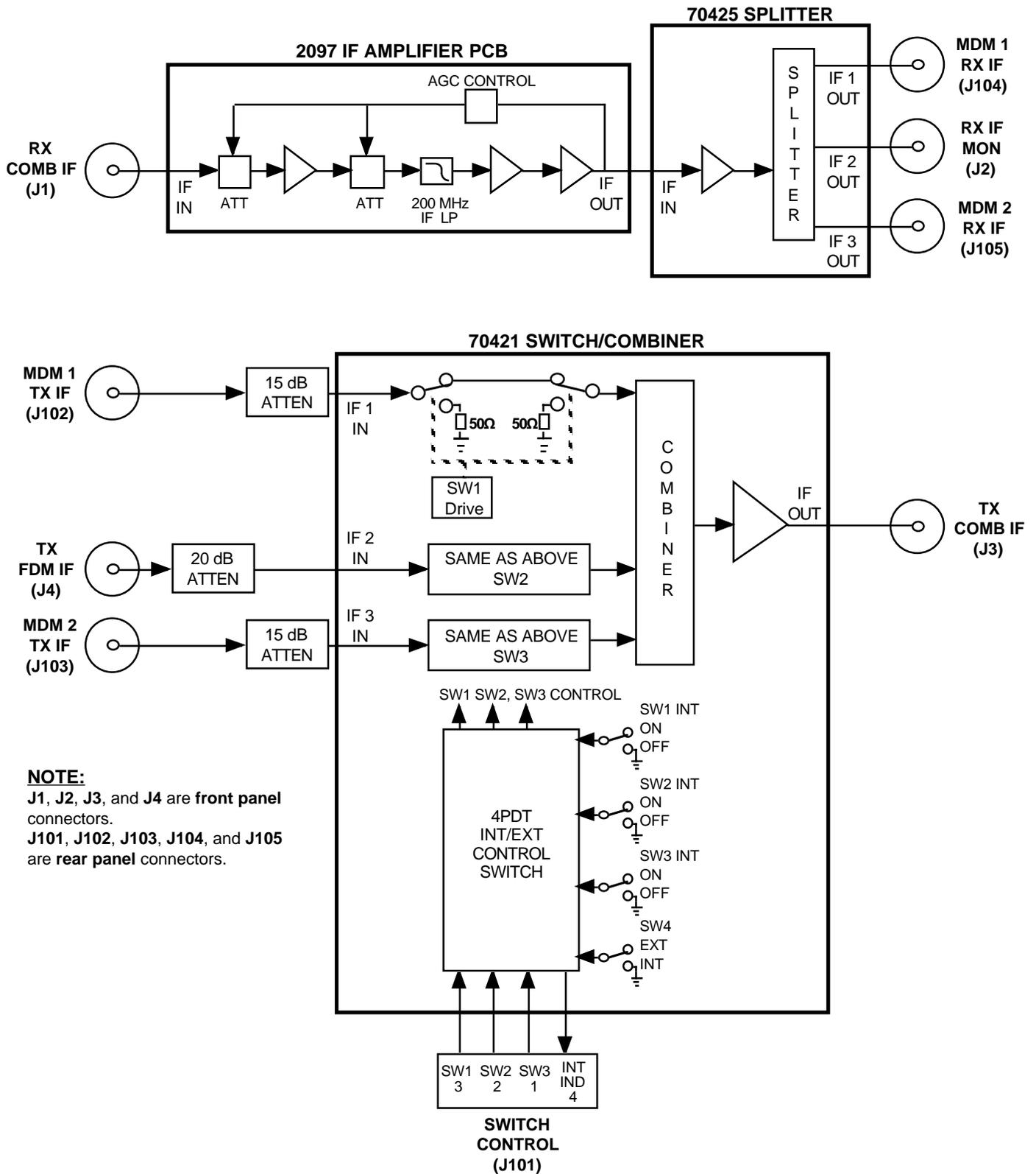
Figure 1:2 Model 1200 Block Diagram
