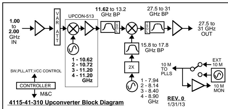
**FIGURE 1.0 Model 4115-41-310 Ka-Band Upconverter Block Diagram**
