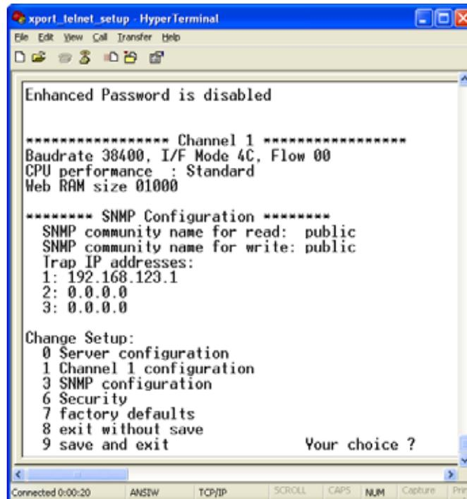
**Figure 3.5: Device Server Configuration Menu**
