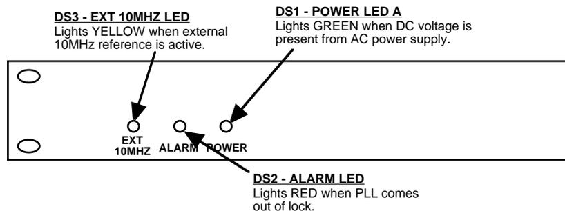
**FIGURE 2.2 2116-184 Front Panel Controls and Indicators**
