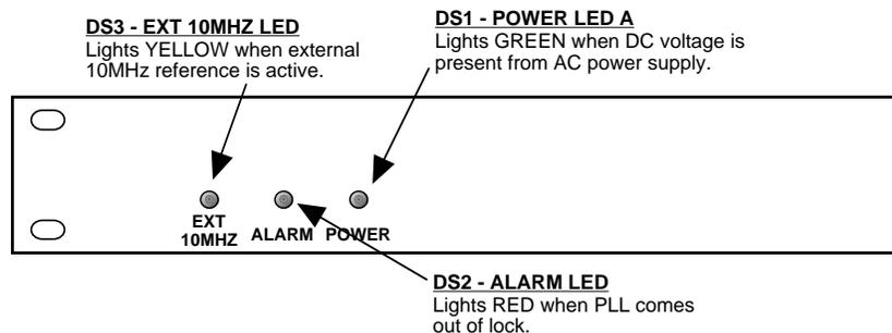
**FIGURE 2.2 2116-137 Front Panel Controls and Indicators**
