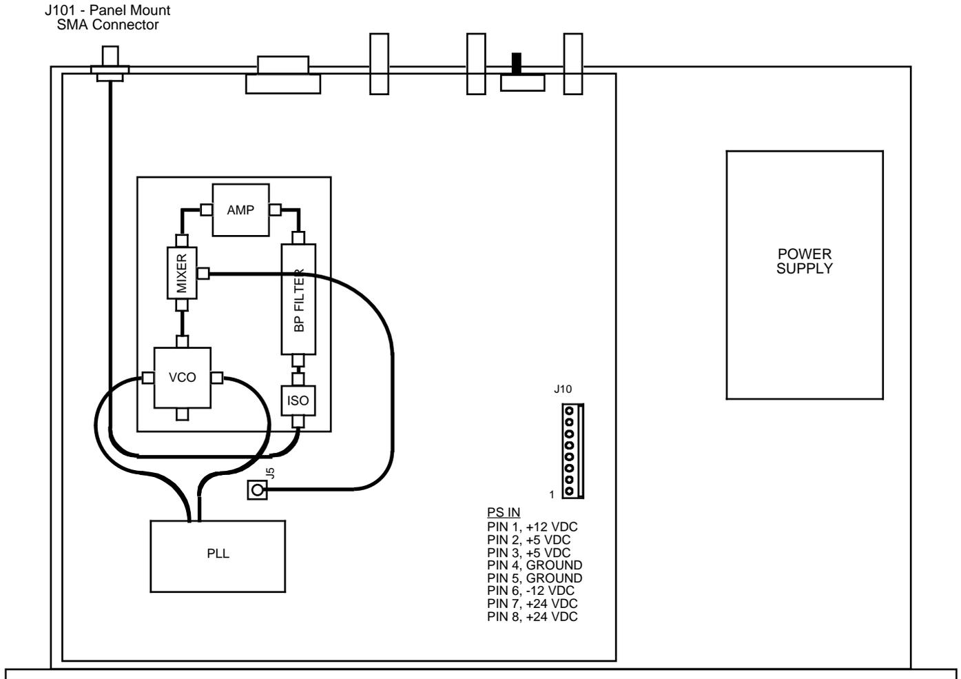
**FIGURE 2.0 2116-137 Mechanical Assembly**
