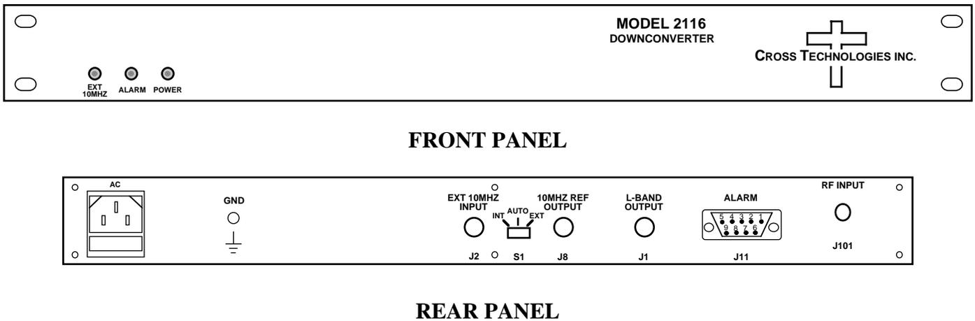
**FIGURE 1.1 Model 2116-137 Front and Rear Panels**
