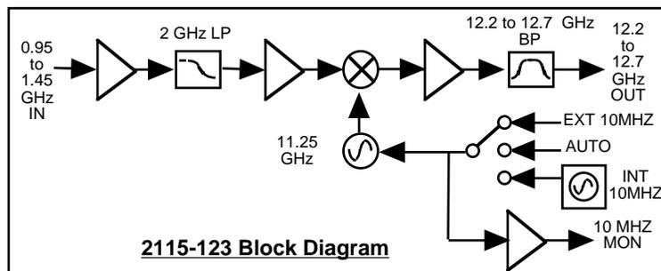
**FIGURE 1.2 Model 2115-123 Upconverter Block Diagram**
