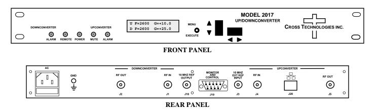
Figure 1.1 Model 2017-2727# Front and Rear Panels
