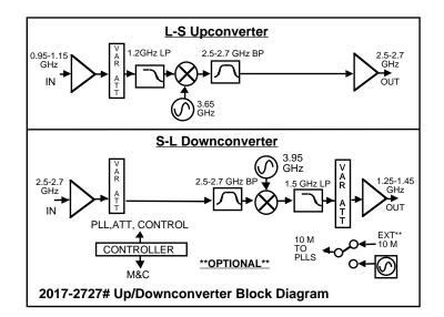
Figure 1.2 Model 2017-2727# Up/Downconverter Block Diagram
