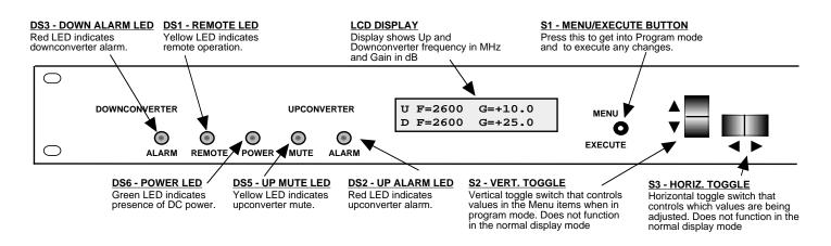
Figure 2.2 Model 2017-2727# Front Panel Controls and Indicators
