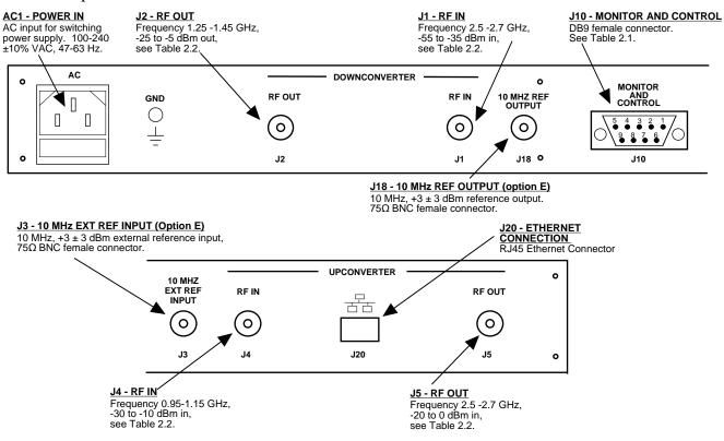
Figure 2.1 Model 2017-2727# Rear Panel I/O's
