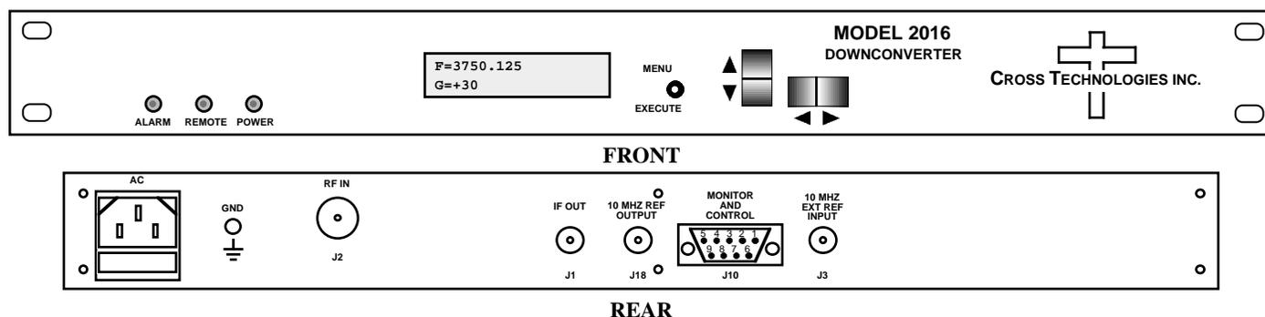
**FIGURE 1.1 Model 2016-34 Front and Rear Panels**
