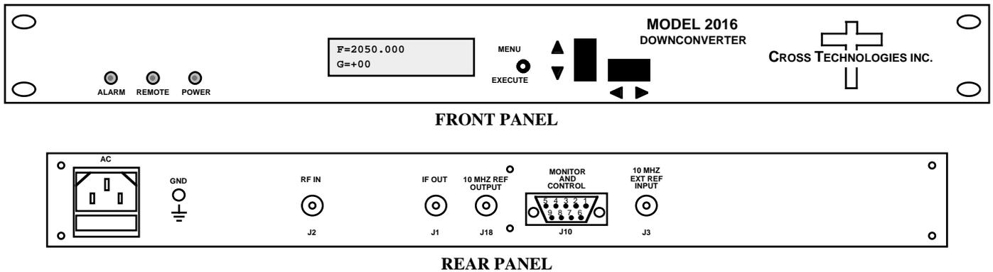
**FIGURE 1.1 Model 2016-225 Front and Rear Panels**
