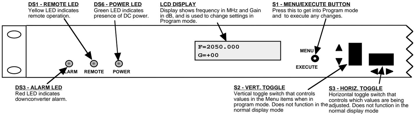
**FIGURE 2.3 2016-225 Front Panel Controls and Indicators**
