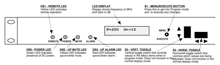
FIGURE 2.3 Front Panel Controls and Indicators
