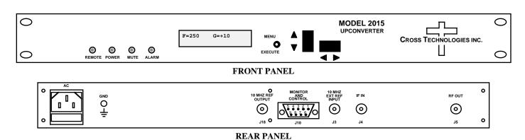
FIGURE 1.1 Front and Rear Panels
