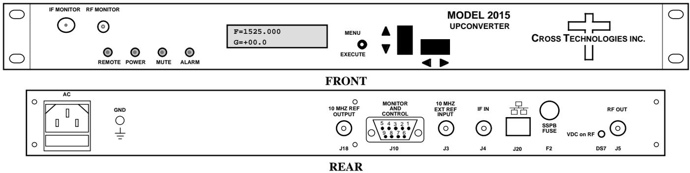
**FIGURE 1.1** Model 2015-24 Front and Rear Panels
