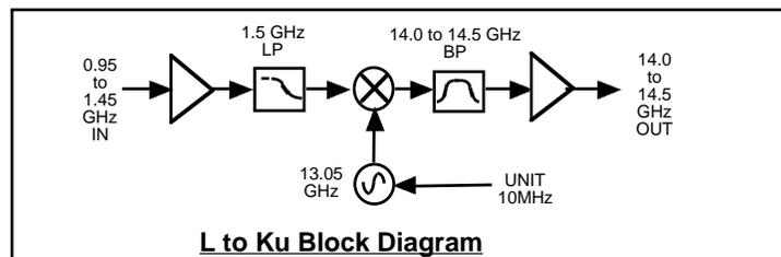
FIGURE 1.3 Model 2015-03U140 L to Ku Block Diagram
