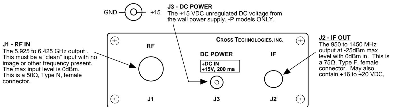
**FIGURE 2.3 Model 2009-59 Rear Panel Inputs and Outputs**
